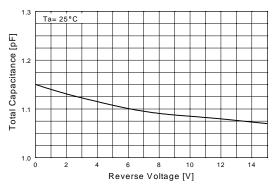
Figure 6. Total Capacitance vs Reverse Voltage
