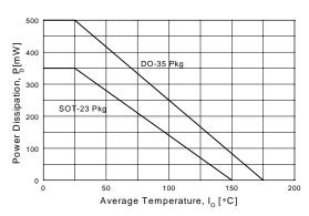
Figure 9. Power Derating Curve
