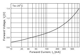
Figure 5. Forward Voltage vs Forward Current VF - 10 - 800 mA
