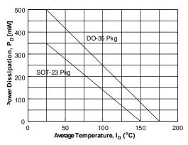
Figrue 9. Power Derating Curve
