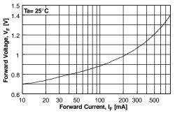
Figure 5. Forward Voltage vs Forward Current VF - 10 - 800 mA
