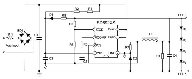
Note: The above circuit and parameters are for reference only; please set the parameters of real application circuit based on real test. SD692XS includes SD692XAS/SD692XBS/SD692XS.
