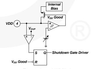
Figure 11. Internal OVP Block
