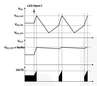
Figure 12. Waveforms in Open-LED Condition
