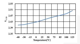
Figure 19. V<sub>CCR</sub> vs. Temperature
