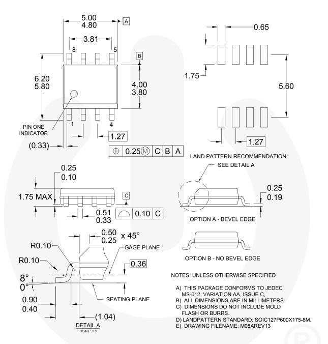
Figure 23. 8-Lead, Small Outline Integrated Circuit Package (SOIC)
