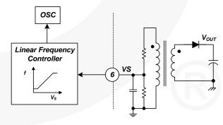
Figure 7. Linear Frequency Control
