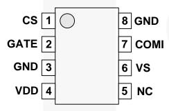
Figure 4. Pin Configuration
