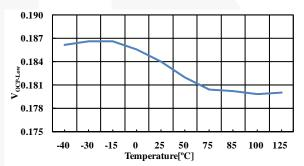
Figure 22. V<sub>OCP-LOW</sub> vs. Temperature
