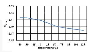
Figure 20. V<sub>VVR</sub> vs. Temperature
