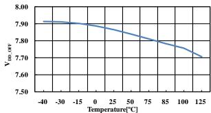
Figure 13. V<sub>DD-ON</sub> vs. Temperature
