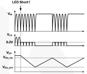
Figure 10. Waveforms in Short-LED Condition
